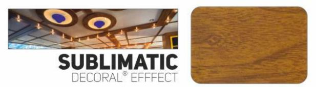
The wood finish Sublimatic Decoral\* Effect is obtained through the sublimation process. The production cycle is divided into several steps, including coating with special polyurethane Powders (Decoral System polyurethane powder coating) and heat transfer, which requires sublimation Films (Decoral System heat transfer films).
